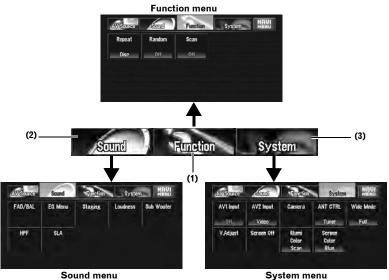
D When the source is "OFF", the "Function" key changes to "Initial" key.
